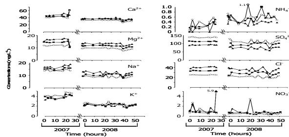
Figure 3. Temporal fluctuations of ion concentrations of the river water following the fire (April 5-6, 2007 and April 5-7, 2008). Closed triangle; P3, Open circle; P4, Closed square; P5.
